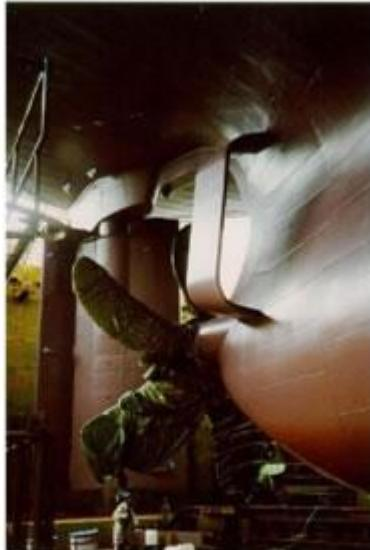
**Figure 6.1 Simple Compensative Nozzle**
