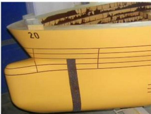
**Figure 17 – Proposed fore body modification for a Tanker conversion project**
