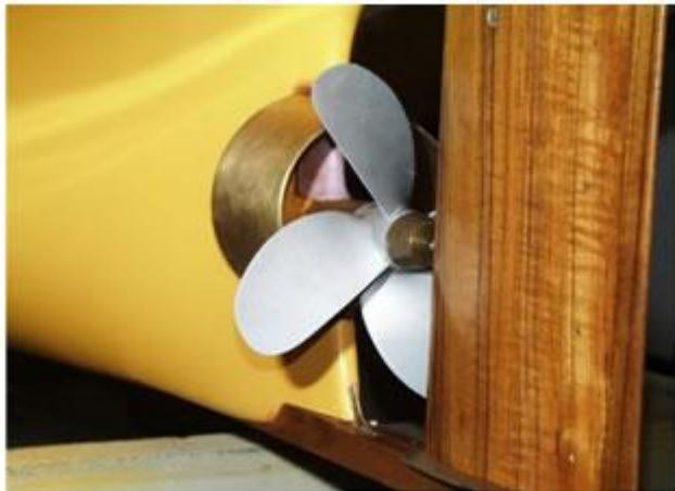
Figure 11 – Sumitomo Integrated Lammeren Duct (SILD)
