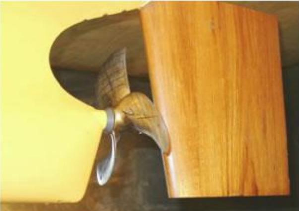
**Figure 13 – VLCC ship model tested with a 3-bladed propeller designed by MMG**
