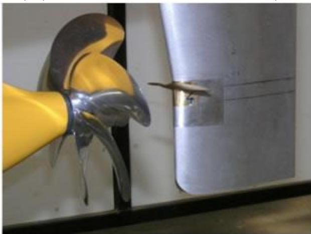
Figure 7 – HHI thrust-fin
