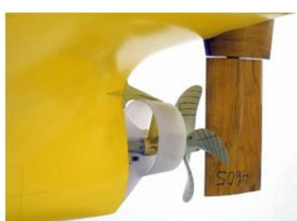
Figure 12 – Bulk carrier model with BMS Mewis Duct®
