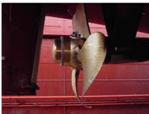
**Figure 4.3 Kappel Propeller
