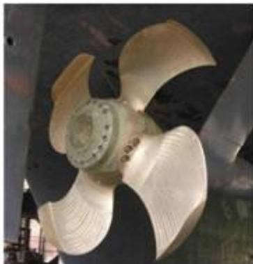
**Figure 4.2 Typical CLT propeller
