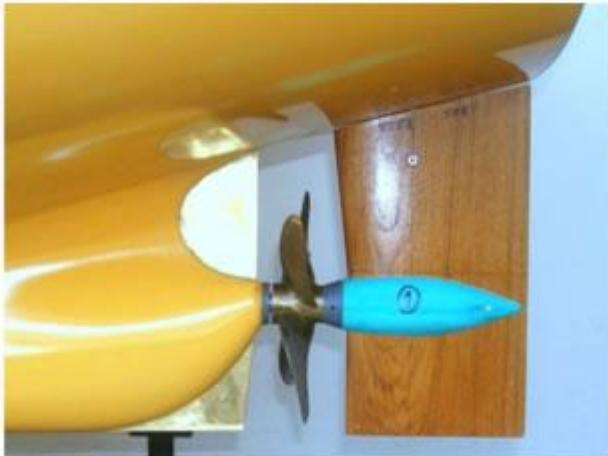
**Figure 16 – Bulk carrier ship model with rudder bulb**
