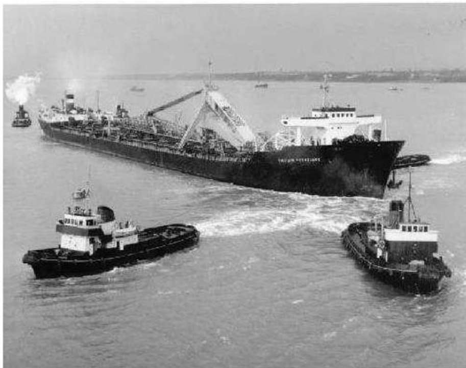
Figure 2.2: Sinclair Petrolore: Self-Unloading Ore-Oil Carrier. Source: www.solentwaters.co.uk
