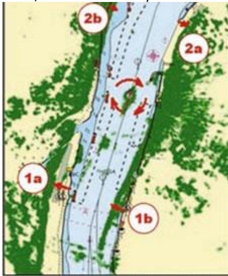
Figure 8 Rotated radar image due to course sensor error
